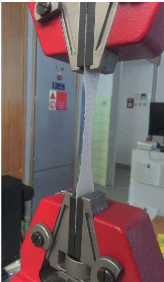
Fig. 1 A specimen clamped in the tensile testing device
