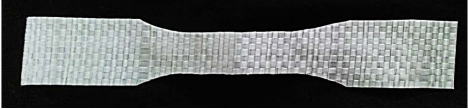
Fig. 2 Example of a specimen geometry, this particular piece is cut in the warp direction
