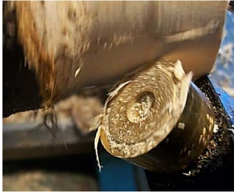
Fig. 18 Turning of wood with rotating bowl-shaped knife
