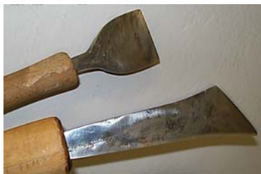
Fig. 2 Original tools for turning at pedal lathe (collection of author)
