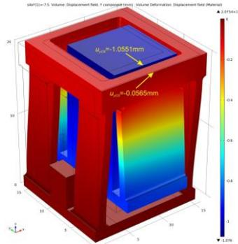
Fig. 5 Displacement of proposed xy sensor in y-direction
