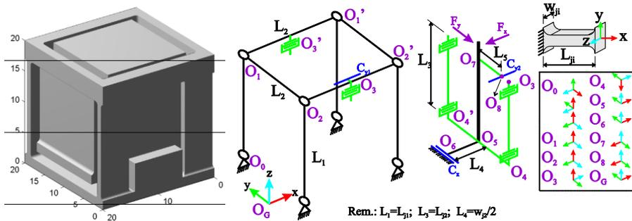
**Fig. 4** Proposed compliant structure of sensor (left), geometry of the final design, and orientation of local coordinate system in observed points
