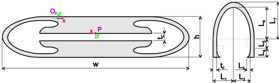
**Fig. 2** Dimensions of deformable part of load cell
