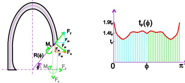
**Fig. 3** The curved beam element with forces and torque distribution (left), dependence of flexure thickness on angle  $\phi$
