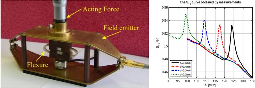
**Fig. 1** Physical model of prototype of novel force/displacement sensor (left), the  $S_{11}$  curve obtained by measurements (right)
