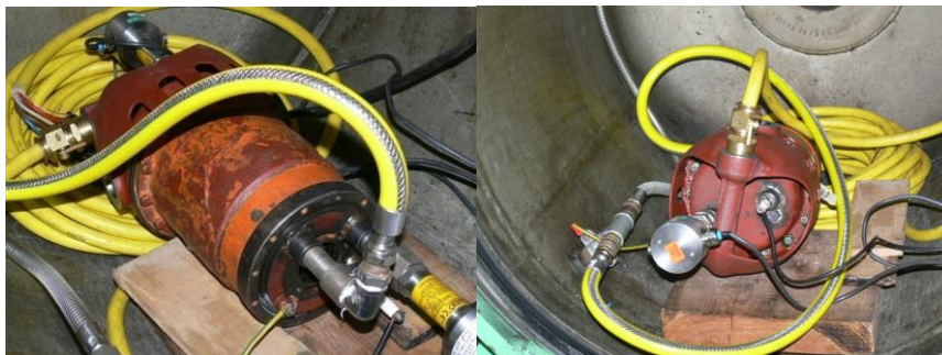
Fig. 22. shows the parts of pumping engine prepared to test flameproof enclosure
