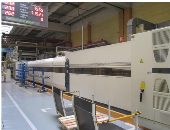
Fig 7. Side view of the drying section of the gluing machine
