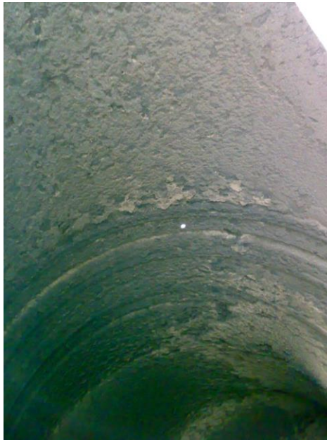
Fig 11. View of the deposits on the inner wall of the exhaust of crimping stool No. 1
