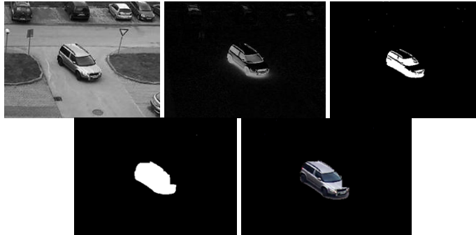
Fig. 5 Processing a moving object in Block4 (from left); original, difference images, thresholding, dilation and erosion, mask
