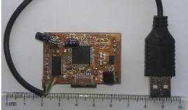
Fig. 3, Fig. 4 Inertial measurement unit used for testing [4]
