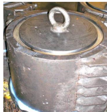
Fig. 1.6 Sintering apparatus with plates prepared for gluing
