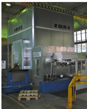
Fig. 2.1 Two-point eccentric press ZDAZ LKD 400
