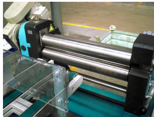
Fig. 3.9 Four-cylinder bending rolls of the production line
