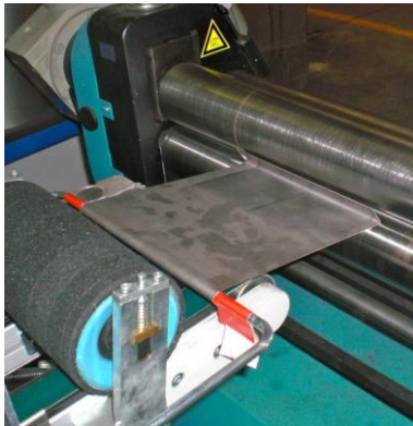
Fig. 3.8 Preparation for direct the strip to the bending rolls
