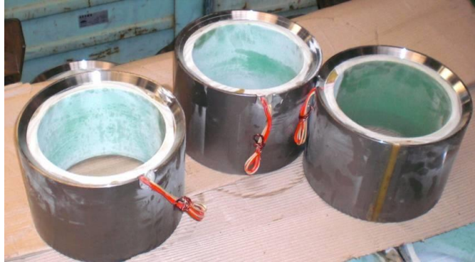
Fig. 1.7 Stators of inductive sensor with winding
