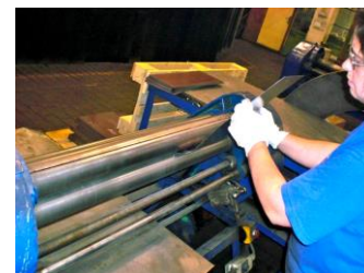
Fig. 2.3 Motor-driven roll bending machine Roundo PAS-360
