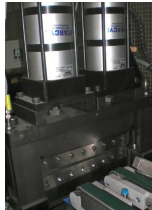
Fig. 3.7 Pneumatic shears with inclined tools
