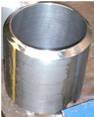
Fig. 1.5 Rotor complex of inductive position sensor
