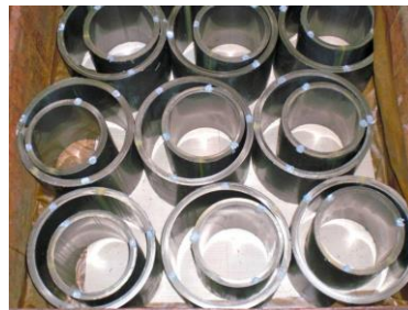
Fig. 2.6 Stator and rotor packets of inductive position sensor
