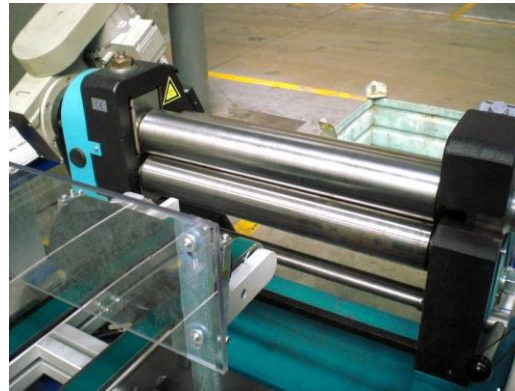
Fig. 3.9 Four-cylinder bending rolls of the production line
