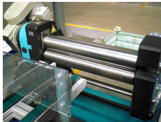
Fig. 3.9 Four-cylinder bending rolls of the production line
