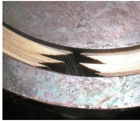
Fig. 2.4 Gap between the ends of roll bended strips before flooding by the two-component epoxy
