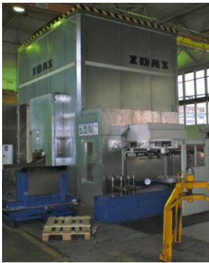
Fig. 2.1 Two-point eccentric press ZDAZ LKD 400
