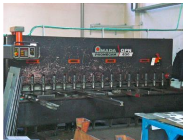
Fig. 2.2 Hydraulic plate shears Amada GPN 630
