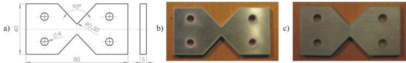
Fig. 1 a) Geometry of the test specimen - „butterfly’s shape“; b) Dural ; c) Stainless steel
