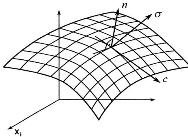
**Fig. 1** Shear stress on general curved surface.
