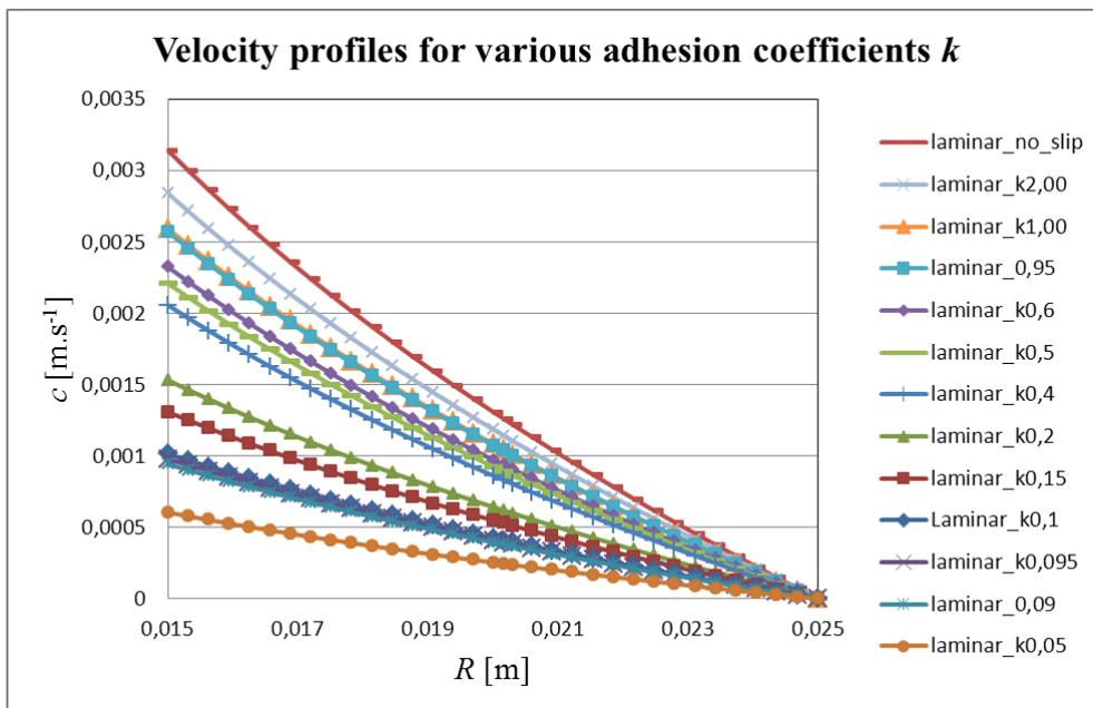
**Fig. 5** Velocity profiles for various adhesion coefficients  $k$  at  $n = 2$  rpm on inner cylinder.
