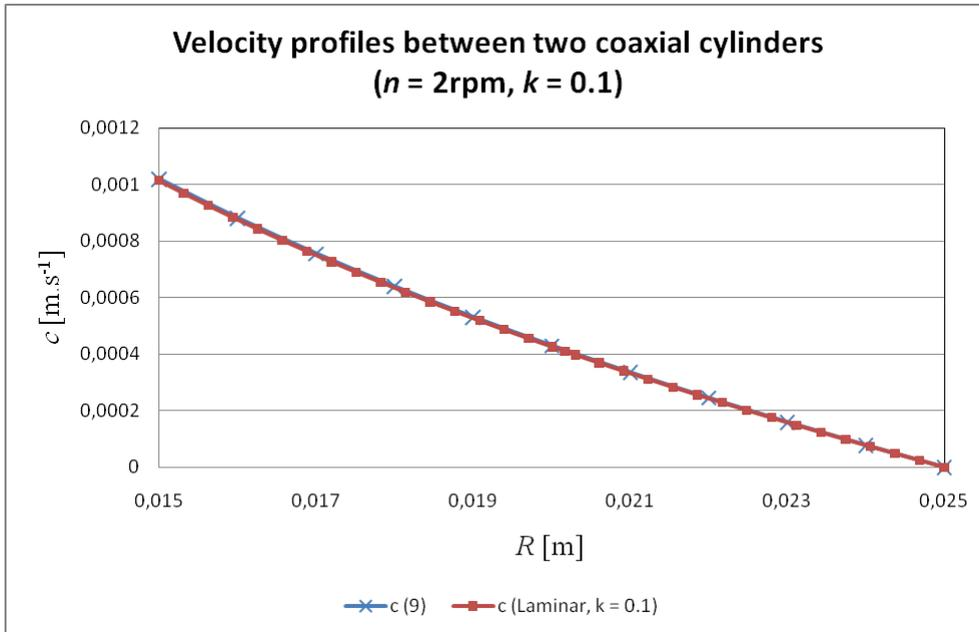
**Fig. 4** Comparison of velocity profiles for  $n = 2$  rpm, inner cylinder is partially wetttable.
