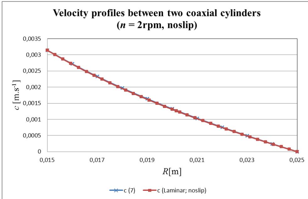
**Fig. 3** Comparison of velocity profiles at  $n = 2$  rpm, inner cylinder is fully wettable.
