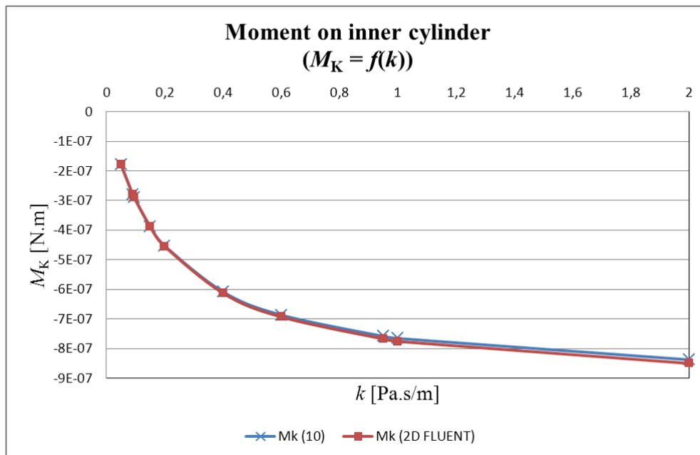
**Fig. 6** Moment is compared on inner cylinder at  $n = 2$  rpm, inner cylinder is partially wettable.
