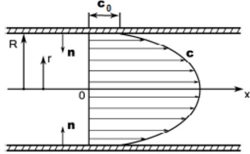
**Fig. 3** Velocity profile for partially wettable surface of the tube.
