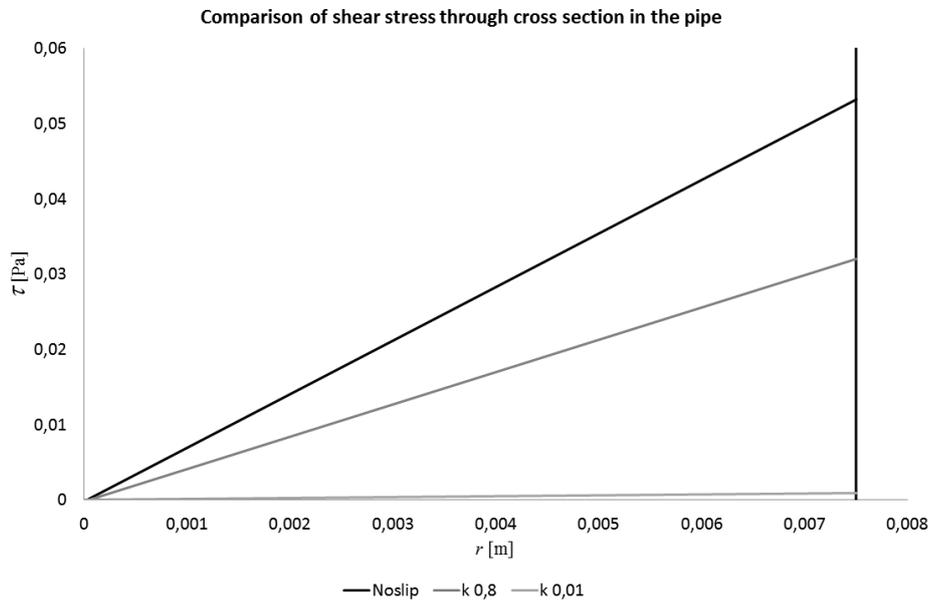
**Fig. 6** Shear stress profile in dependence on  $k$ .
