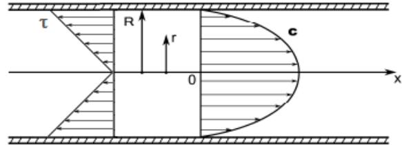
**Fig. 2** Straight pipe section with shear and velocity distribution in case of fully wettable wall (no slip).
