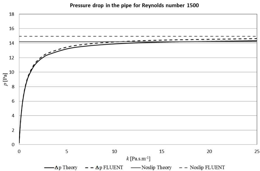
**Fig. 5** Comparison of pressure drop for wettable (no slip) and partially wettable (slip) boundary conditions on the pipe wall for  $Re = 1500$ .
