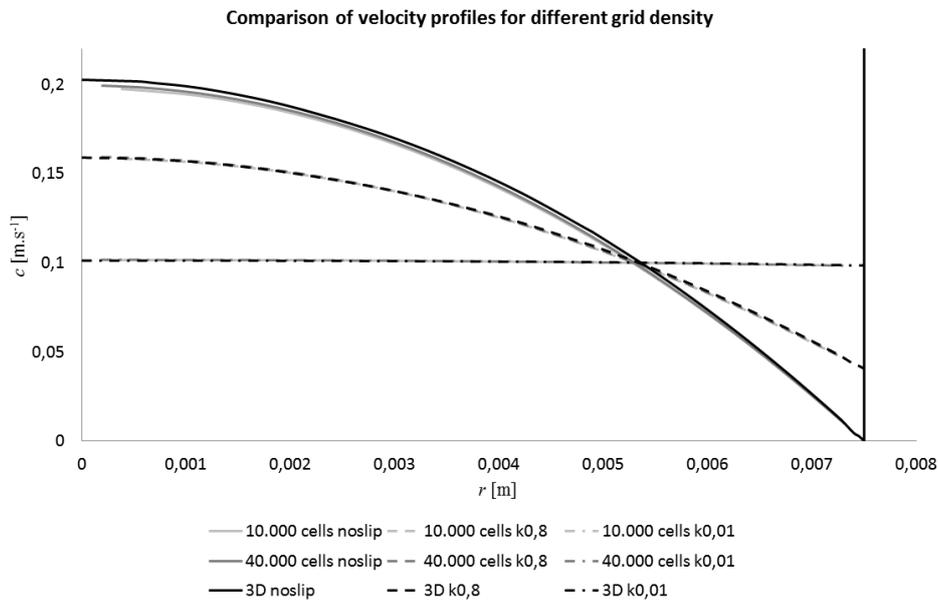
**Fig. 7** Comparison of calculated velocity profiles from 2D and 3D geometry.
