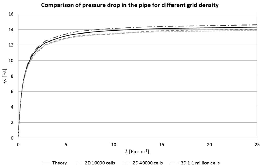
**Fig. 8** Calculated pressure drop in 2D a 3D geometry with different grid density.
