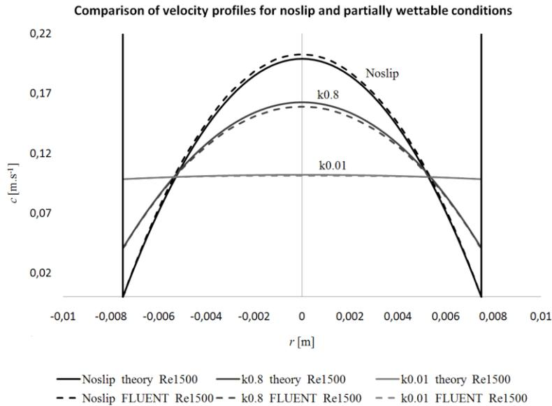
**Fig. 4** Comparison of velocity profiles obtained from theory and FLUENT simulation.
