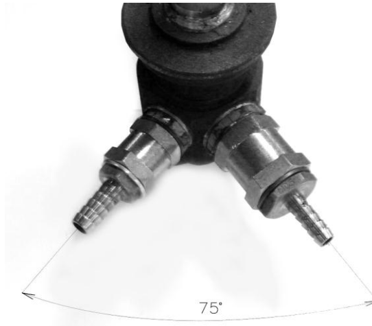
Fig. 3 Detail of burner inputs.
