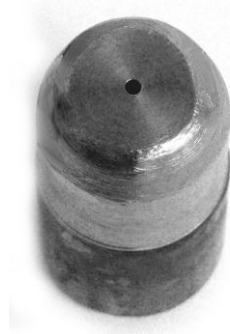
Fig. 5 Modified burner head with one nozzle with diameter 2 mm.
