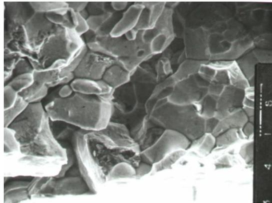
**Fig. 6** Denuded surface of corrosion crack on the blade base.
