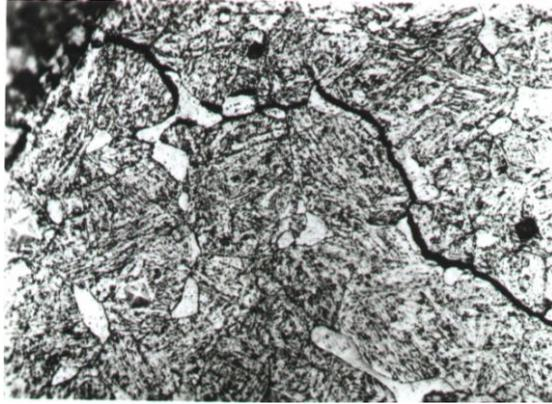
**Fig. 5** The outset of the corrosion crack found on the blade base.
