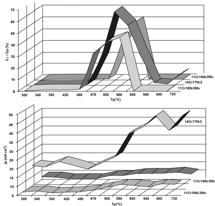
**Fig. 8** Effect of tempering temperature on the coulombic ratio (top) and on the critical passivation current density (bottom) for martensitic stainless steels quenched at 1040°C. Scanned in 0.5M  $H_2SO_4$  + 0.01% KSCN at laboratory temperature and 9 V/h scan rate.
