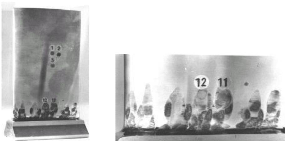
**Fig. 3** Corrosion and fatigue damage on rotor blade indicating EPR test locations: view of blade (left) and detailed view of blade base (right).
