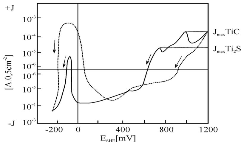
**Fig. 1** Reverse scans of double loop polarization curves for annealed grade Cr18Ni12Ti steel in 2.5M H<sub>2</sub>SO<sub>4</sub>. — 1150°C/20 min/water +590°C/20 h/water
