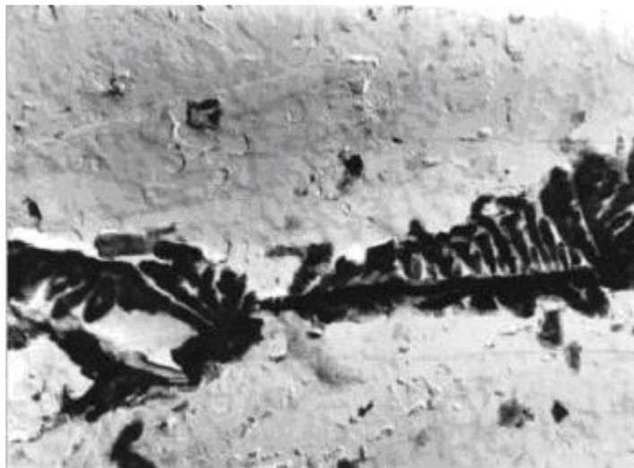
**Fig. 4** Extraction thin foil with precipitated carbides (5000x).
