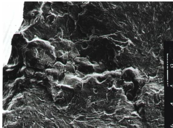
**Fig. 7** Starting point of propagation of a fatigue crack on the facets
