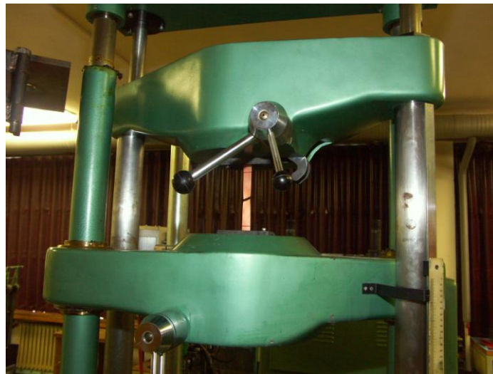
Fig. 5 Tensile testing machine with tensile specimen after test.
