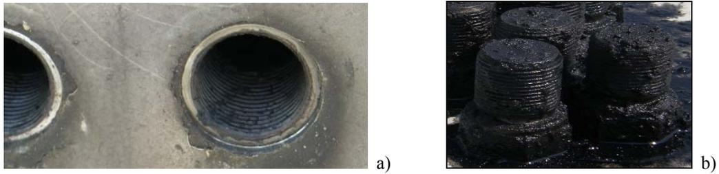
**Fig. 1** a) Clean inside surface at the inlet section of the gas collector
