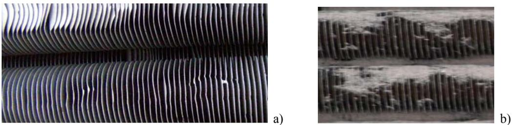
**Fig. 2** a) Detail of clean outside heat transfer surface
