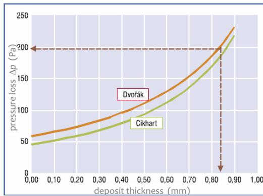
**Fig. 8** Pressure loss as depending on the cleanness of the outside heat transfer surface
