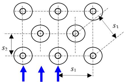
**Fig. 3** The arrangements of tubes
