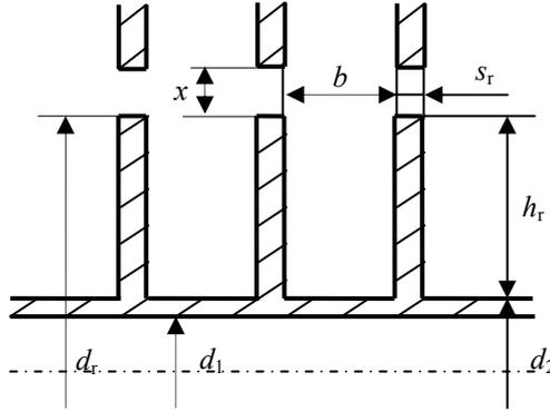
**Fig. 5** Geometry of heat transfer surface of the pipe in the cooler
