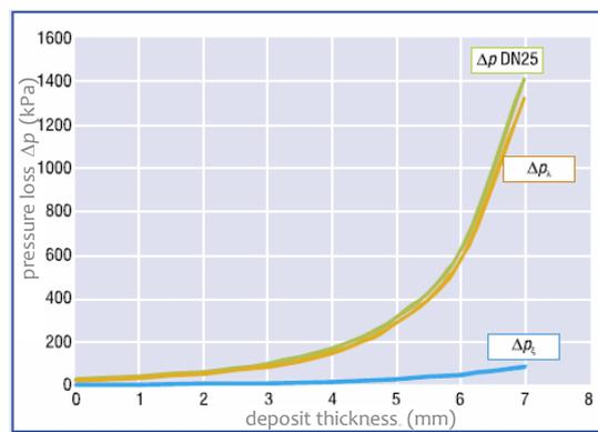
**Fig. 9** Pressure loss as depending on the cleanness of the inside heat transfer surface
