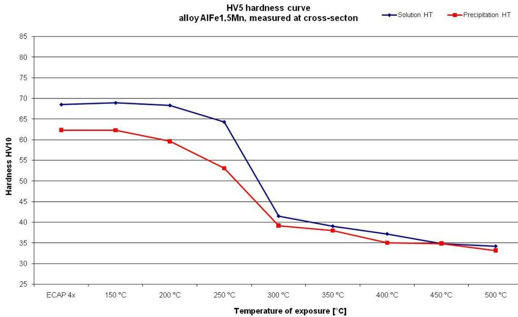
**Fig. 10:** Determination of a critical temperature of AlFe1,5Mn, note: S – solution annealing, T - precipitation annealing
