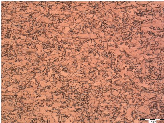
**Fig. 5a:** Microstructure of Cu 99,5 in an initial state, transverse direction, mag. 100x, scale 100 μm
