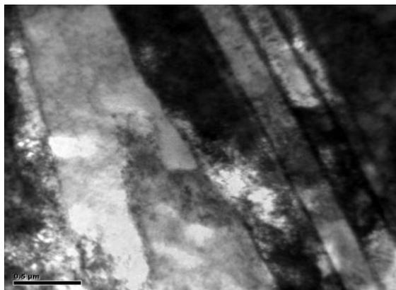
**Fig. 6:** TEM of Cu 99,5 after 6<sup>th</sup> pass, , scale 0,5 μm α brass
