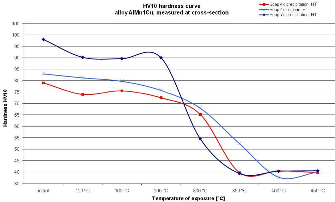
**Fig. 11:** Determination of a critical temperature of AlMn1Cu, note: solution annealing, precipitation annealing, 4x, 7x - number of passes
