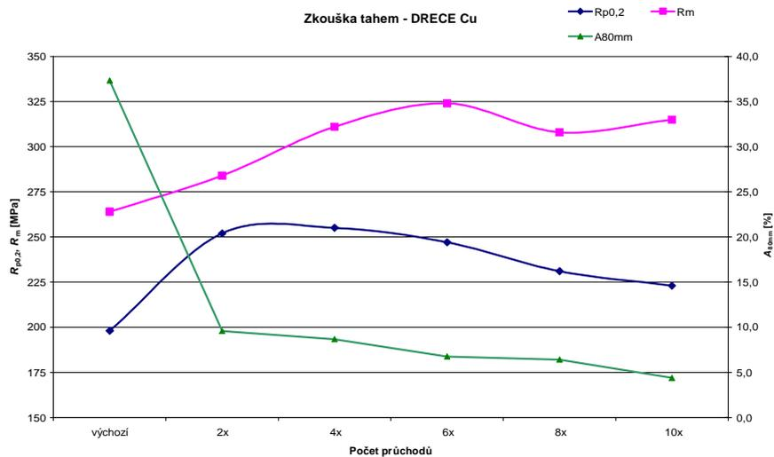
**Fig. 8:** Influence of pass number on mechanical properties of Cu 99,5 (tensile test at ambient temperature)
