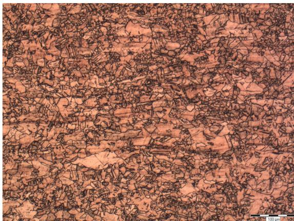
**Fig. 5b:** Microstructure of Cu 99,5 after 8<sup>th</sup> pass, transverse direction, mag. 100x, scale 100 μm
