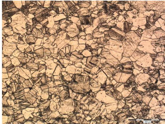
**Fig. 7b:** Microstructure of alpha brass after 4<sup>th</sup> pass, transverse direction, mag. 100x, scale 100  $\mu\text{m}$
