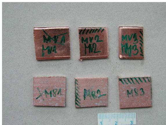
**Fig. 4:** Macro photo of Cu 99,5 in an initial state and after 8<sup>th</sup> pass
