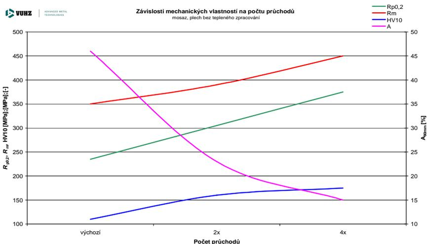
**Fig. 9:** Influence of pass number on mechanical properties of alpha brass (tensile test at ambient temperature, Vickers hardness)
