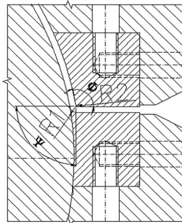
**Fig. 2a:** Original geometry of DRECE forming tool
