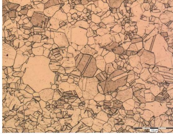
**Fig. 7a:** Microstructure of alpha brass in an initial state, transverse direction, mag. 100x, scale 100  $\mu\text{m}$
