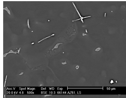
Fig. 2 Structure of as-cast alloy AZ61 (SEM)
