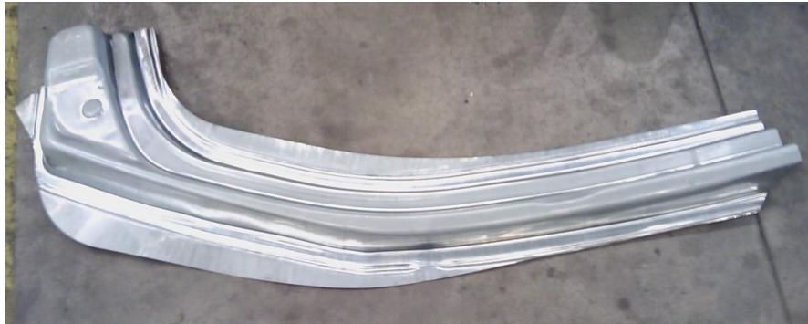
Fig. 1 Inside reinforcement of the car front door
