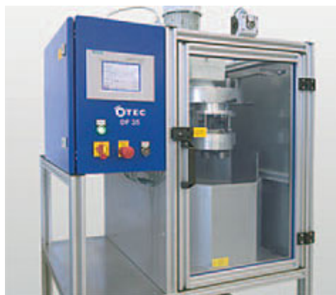
Fig. 5 Tumbling Machine OTEC DF 35
