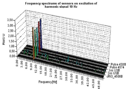
**Fig. 7** Frequency spectrums on measurement harmonic signal 10 Hz
