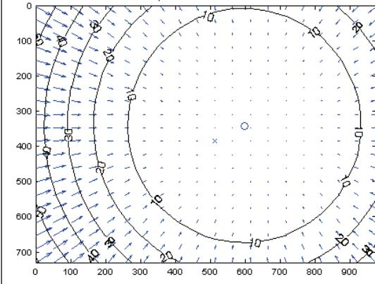
**Figure 2** Left camera radial lens distortion
