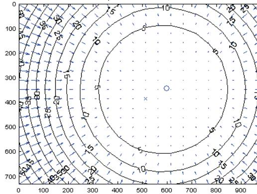
**Figure 4** Complete model of the left camera lens distortion
