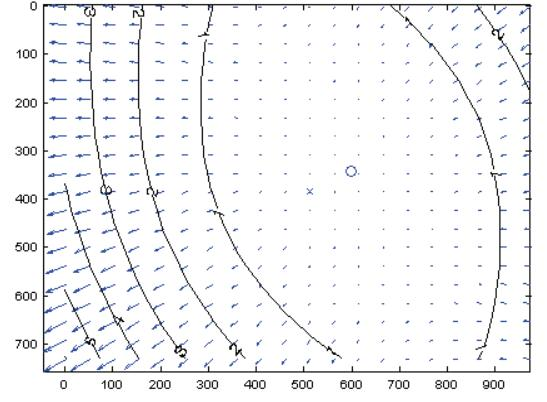
**Figure 3** Left camera tangential lens distortion
