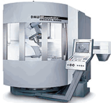
Fig. 1 The universal DMU 60 monoBLOCK® cutting center [6]
