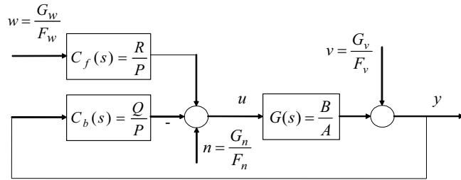
**Fig. 5** 2DOF control system configuration
