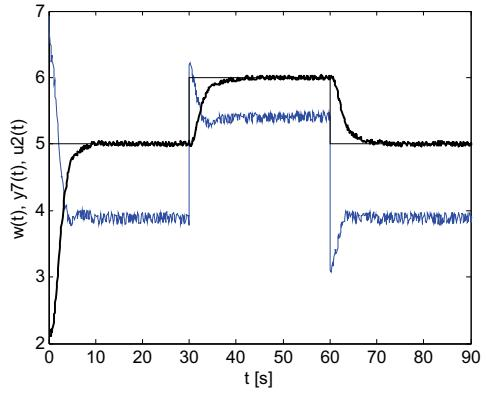
**Fig. 7** Control of airflow speed by regulator (15)
