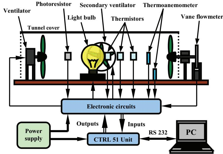
**Fig. 1** Diagram of hot-air model and control system
