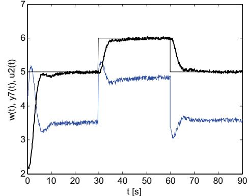
**Fig. 10** Control of airflow speed by regulator (19)
