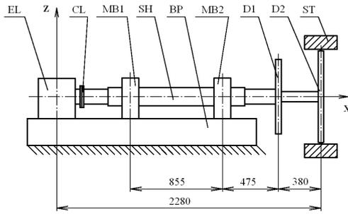
**Fig. 2** Scheme of the rotor system
