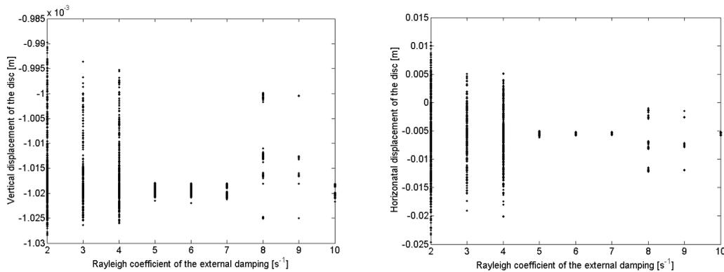
**Fig. 3** Bifurcation diagram based on vertical (left) and horizontal (right) displacement of the centre of the disc D2
