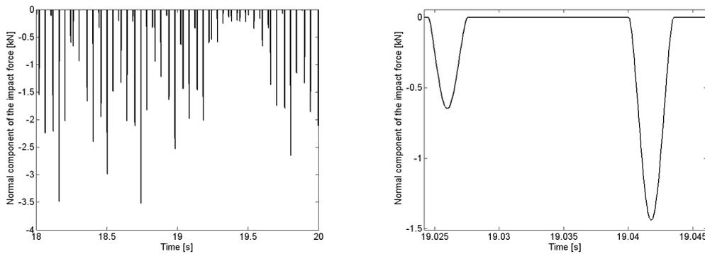
**Fig. 8** Normal component of the impact force (left) and the detail its time history (right)
