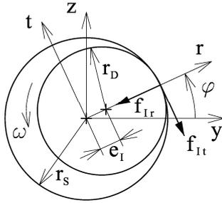
**Fig. 1** Scheme of the impact between the disc and the stationary part
