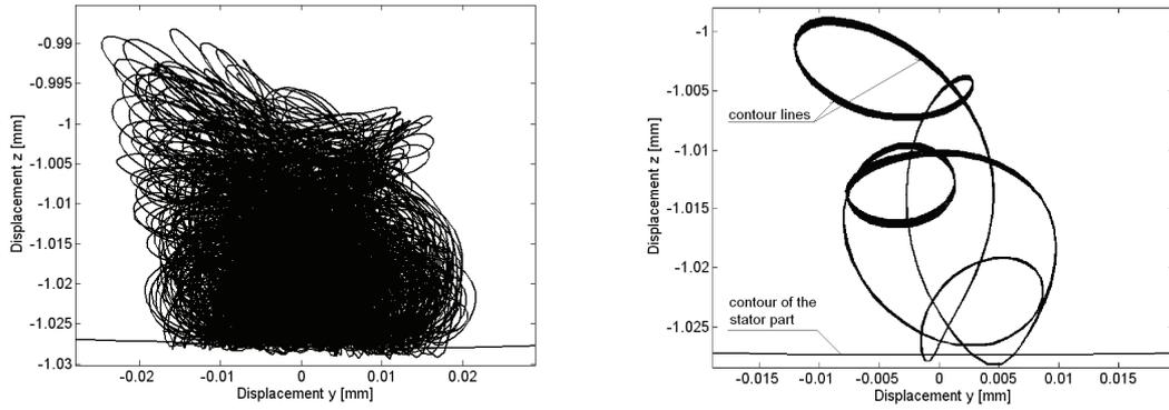
**Fig. 4** Steady-state orbit of the centre of the disc D2 for magnitude of Rayleigh coefficient of external damping  $\alpha=2s^{-1}$  (left) and  $\alpha=8s^{-1}$  (right)
