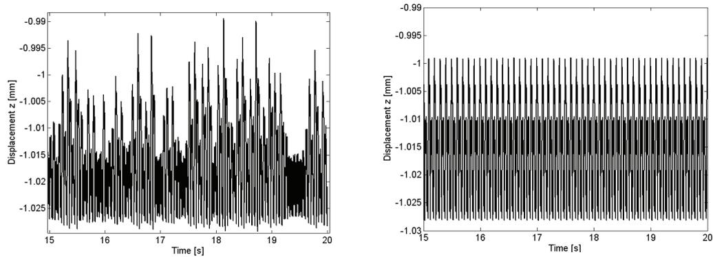
**Fig. 6** The time history vertical displacement of the centre of the disc D2 in the steady-state of the rotor system for magnitude of Rayleigh coefficient of external damping  $\alpha=2s^{-1}$  (left) and  $\alpha=8s^{-1}$  (right)
