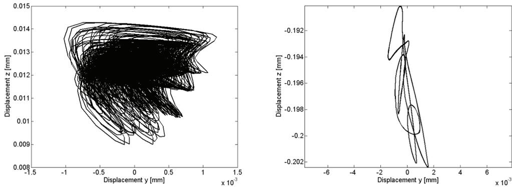
**Fig. 5** Steady-state orbit of the centre of the magnetic bearing MB2 for magnitude of Rayleigh coefficient of external damping  $\alpha=2s^{-1}$  (left) and  $\alpha=8s^{-1}$  (right)
