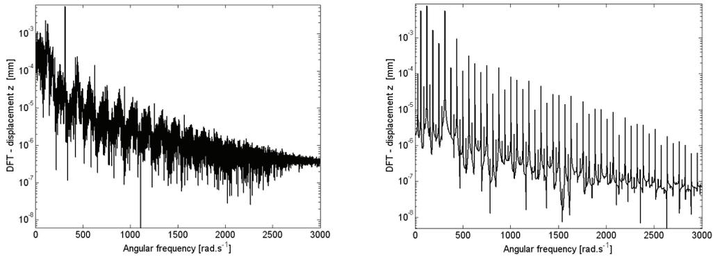
**Fig. 7** Fourier spectra of the steady-state response for magnitude of Rayleigh coefficient of external damping  $\alpha=2s^{-1}$  (left) and  $\alpha=8s^{-1}$  (right)
