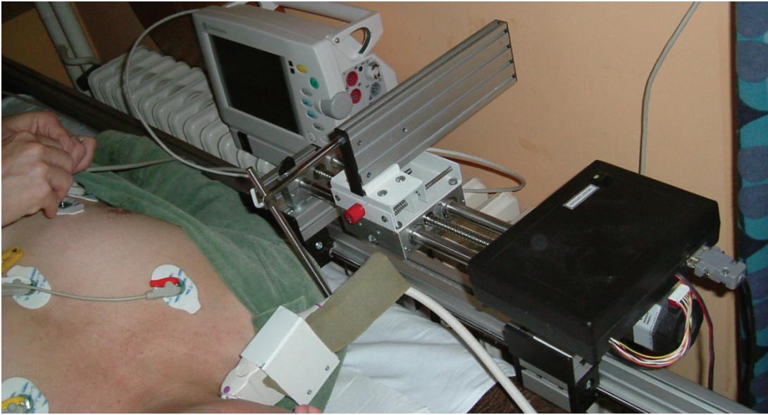
**Fig. 2** Ultrasonic probe linear movement system
