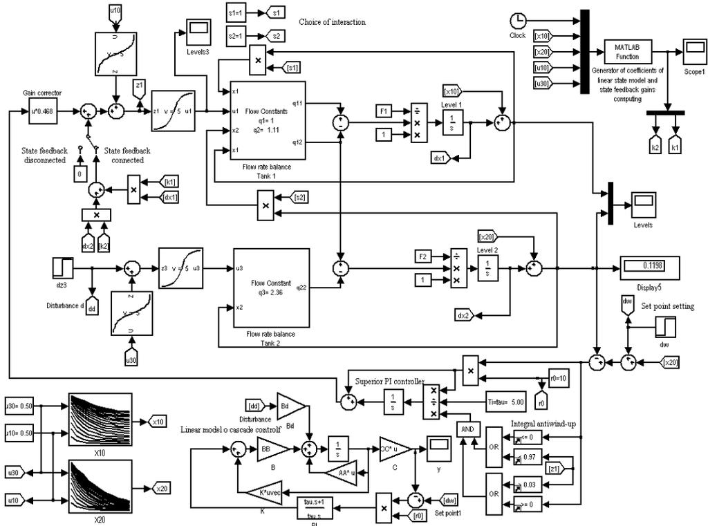
**Fig. 2** Model of tank cascade control in Simulink, including auxiliary linear state model
