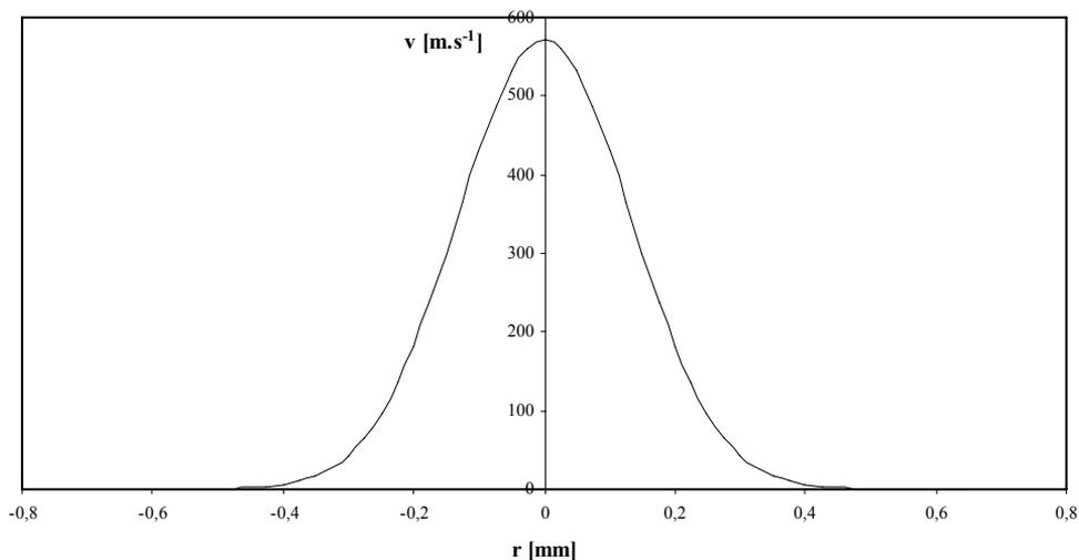
Fig. 2 Velocity field of high-pressure jet in its cross-section 89 mm from the nozzle
