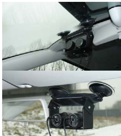
Fig. 6 Camera subsystem with polarized filters
