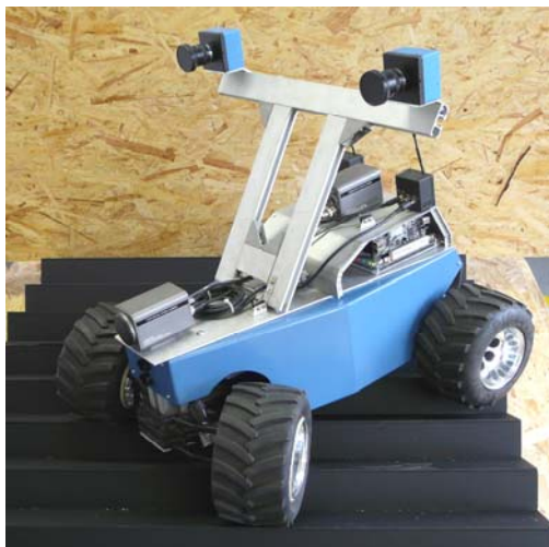
Fig. 2 Prototype of four wheels robot for 3D data capture
