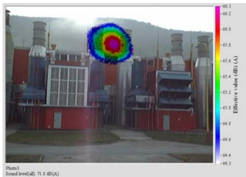
Fig. 7: Visualization of the noise emission intensity by depressurization
