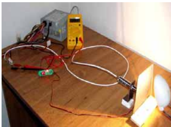
Fig. 11 Photo of measurement stand for testing of non contact sensor with thermocouple detector OMEGA
