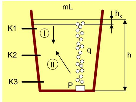
**Fig. 1** Blowing of argon into the ladle model
