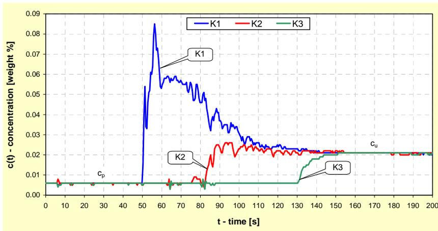
**Fig. 2** Development of concentration in the sensors  $K1$ ,  $K2$  and  $K3$
