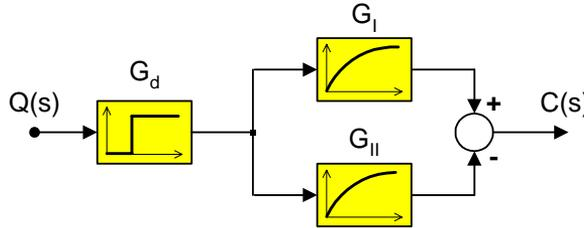
**Fig. 3** Block diagram of the ladle model
