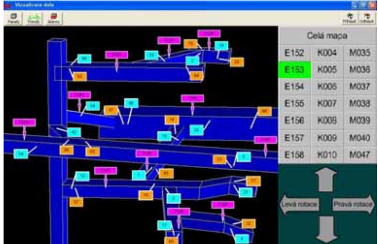
Fig.2 3D display of mine system in Promotic HMI software
