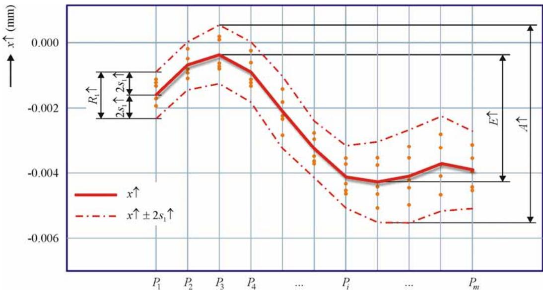
**Fig. 1** Example of the graphical presentation of evaluated positional deviation according to the standard [1] (results plotted for unidirectional positioning)
