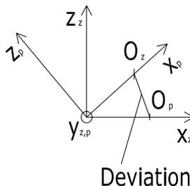
Fig. 4 The showing deviation for point O when there is rotation about axis Y
