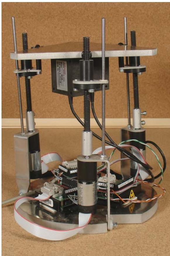
Fig. 5 The realized stabilized platform
