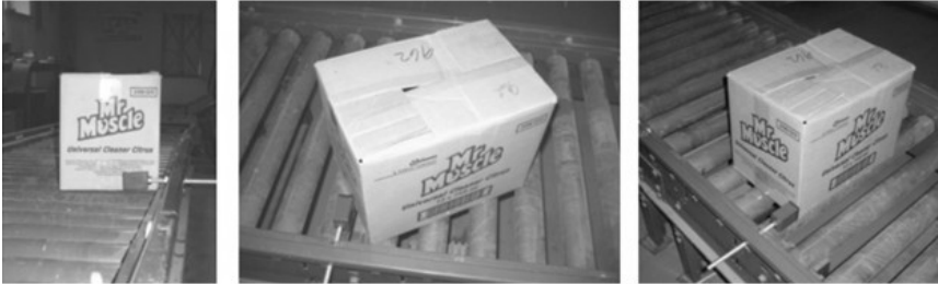
Fig. 10 Transport and handling (turning) of storage crate on roller conveyor
