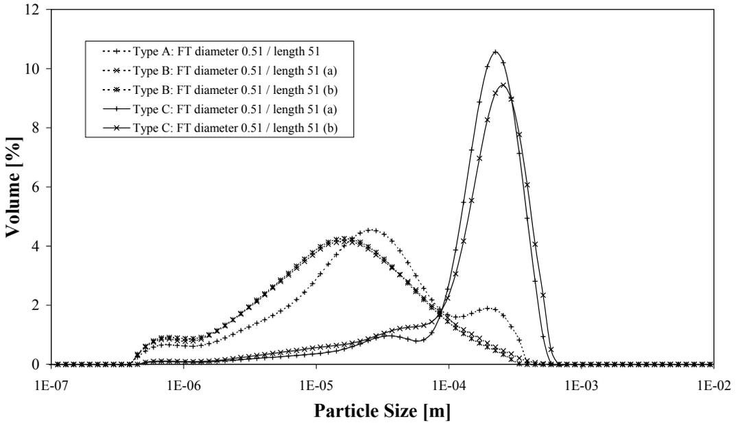
**Fig. 8.** Experimental results of determination of the volume percentage of particle size for heads A, B (diameter of water nozzle of 0.25 mm, pressure of 400 MPa) and C (diameter of water nozzle of 0.15 mm, pressure of 400 MPa) with the focusing tubes (FT) with the same diameter and the length.
