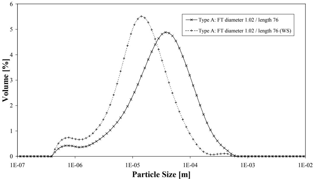
**Fig. 9.** Experimental results of determination of the volume percentage of size of particles got with or without water spraying (WS) under otherwise equal conditions.
