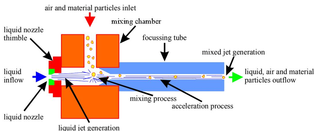
**Fig. 1.** A diagrammatical section through the cutting head of abrasive water jet with the representation of processes leading to the generation of abrasive liquid jet at its exit.
