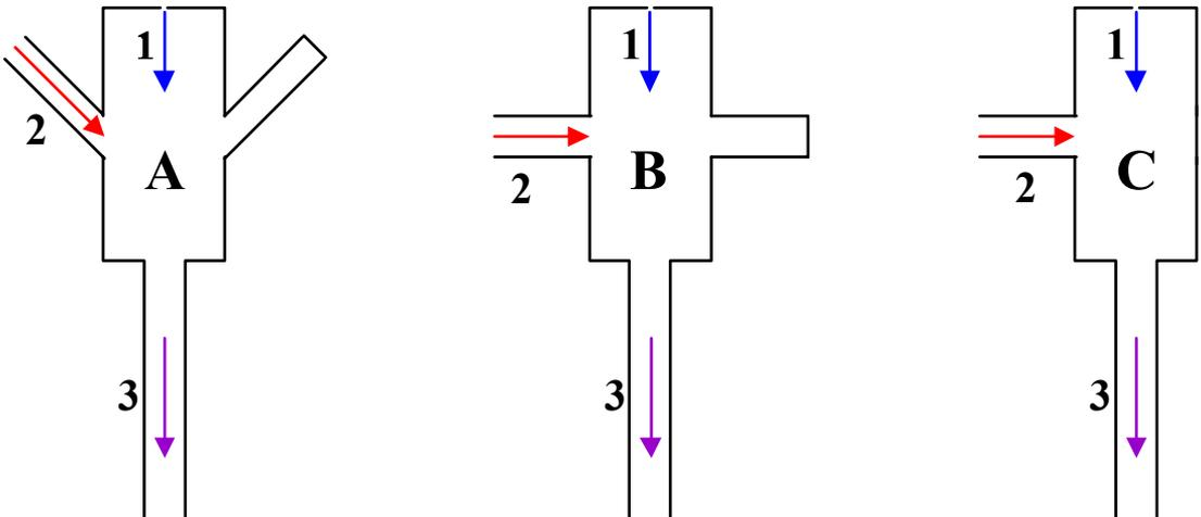
**Fig. 3.** Diagrammatical sections through various configurations of mixing chambers used for the generation of abrasive water jet: 1 – water jet; 2 – mix of sucked air and material particles; 3 – outflow of the mixed jet; A, B, C – mixing chamber configurations.
