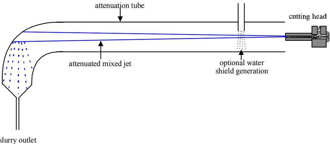
**Fig. 4.** A diagram of experimental set-up at the interception of (abrasive) mixed liquid jet.
