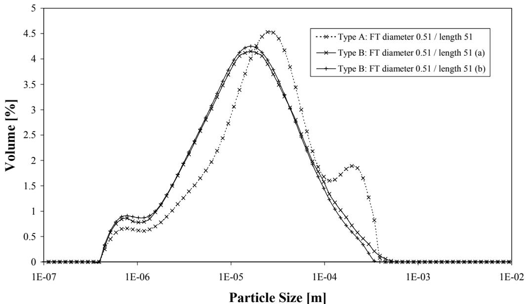
**Fig. 7.** Experimental results of determination of the volume percentage of particle size for various mixing heads (A, B) at the diameter of water nozzle of 0.25 mm, pressure of 400 MPa and the focusing tube (FT) with the same inner diameter and length.
