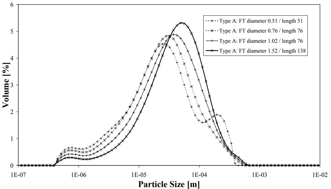
**Fig. 6.** Experimental results of determination of the volume percentage of particle size for the mixing head of type A and the focusing tubes (FT) of various diameters and lengths at the constant diameter of the water nozzle of 0.25 mm and the pressure of water ahead of the water nozzle of 400 MPa.
