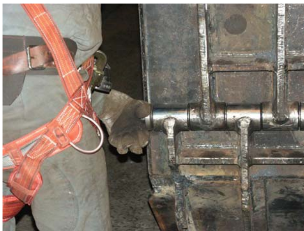
Fig. 6 Blocking of two container parts
