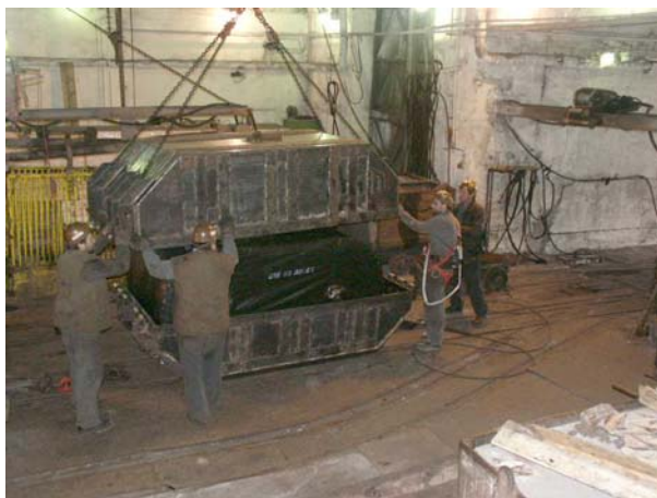
Fig. 5 Fill up and covering two-rolls of transport belt
