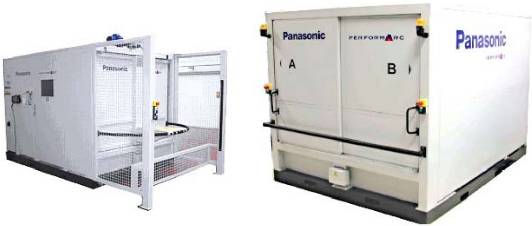
Figure 2: Welding cells Panasonic PerformArc ET and PerformArc TT
