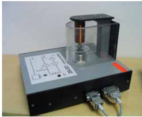
Fig. 2 Model of levitation in magnetic field
