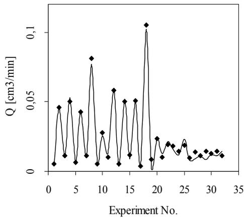
**Fig. 2** Graph between experimental (◆) and predicted values for stock removal (—)
