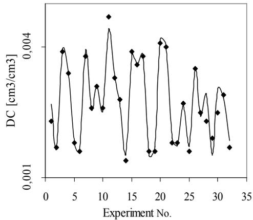
**Fig. 3** Graph between experimental (◆) and predicted values for diamond consumption (—)
