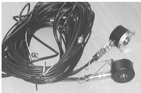
Fig. 5. Heidehain encoders of the ERN 460-500 type (500 pulses per revolution)
