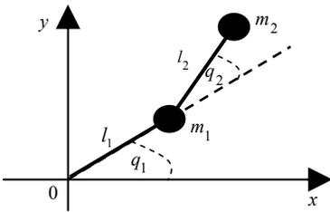
**Fig. 1.** Two degree-of-freedom robot arm
