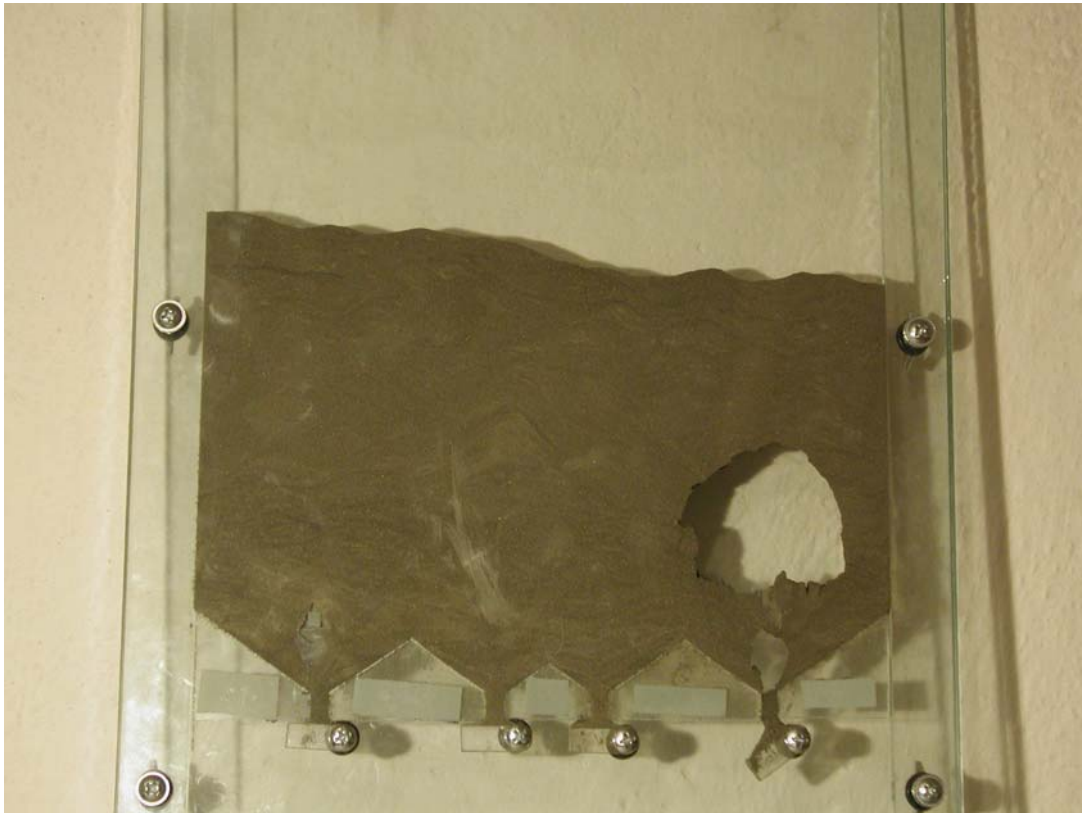
Figure 2 Simulation of the static and the dynamic vault above an outlet opening for the flow of clinker; a situation prior a drop of a static vault [7], VŠB - Technical University of Ostrava, 2004
