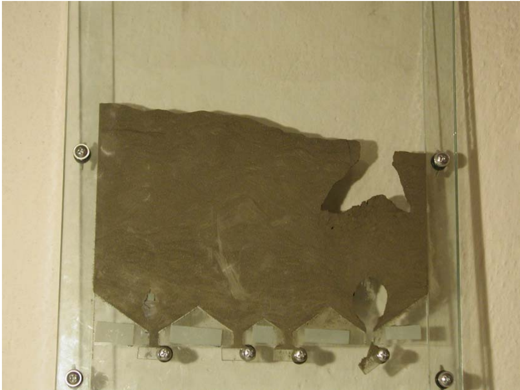
Figure 3 Simulation of the static and the dynamic vault above an outlet opening for the flow of clinker; a situation after the drop of the static vault [7], VŠB - Technical University of Ostrava, 2004
