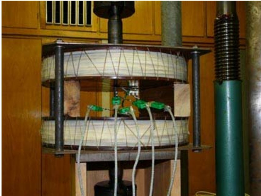
Fig. 4 The sample with welded thermocouples placed in coils, ready for tensile test.
