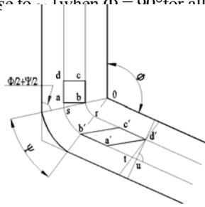
Fig. 4 Principle of equal – channel angular pressing where  $\Phi$  is the angle of intersection of the two channels and  $\Psi$  is the angle subtended by the arc of curvature at the point of intersection.
