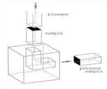
Fig.1 Schematic illustration of ECAP technology
