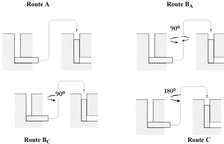
Fig. 2 The four processing routes in ECAP
