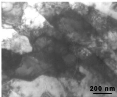
Fig. 7 Structure after the fourth passage by the ECAP tool in AlCu4Mg2 alloy (middle of the sample)
