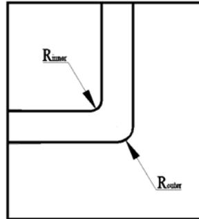
Fig. 9 Inner and outer radius of ECAP tool
