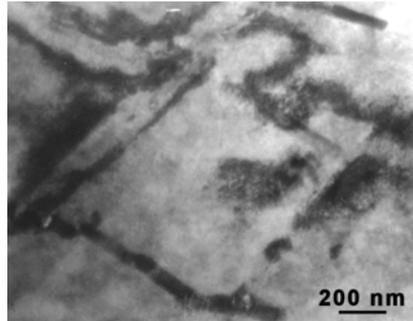
Fig. 6 Structure after the first passage by the ECAP tool in AlCu4Mg2 alloy (middle of the sample)
