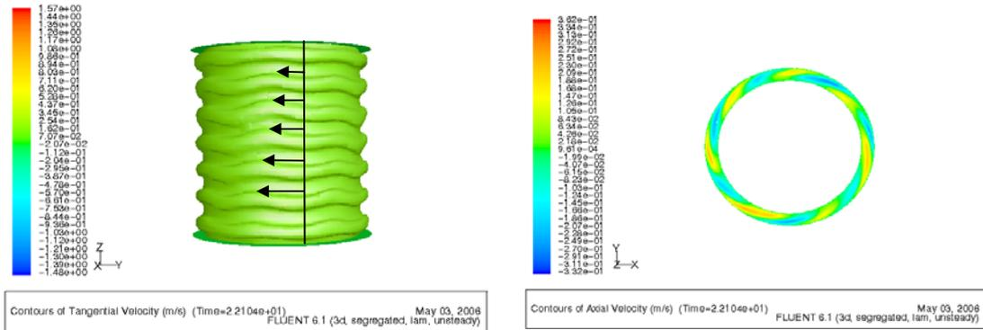
Fig. 4.4 Modulated wavy vortex flow
