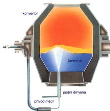
Fig. 1.1 – Oxygen converter with bottom blowing
