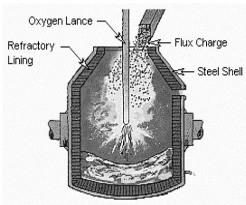
Fig. 1.2 – Oxygen converter with blowing on the surface
