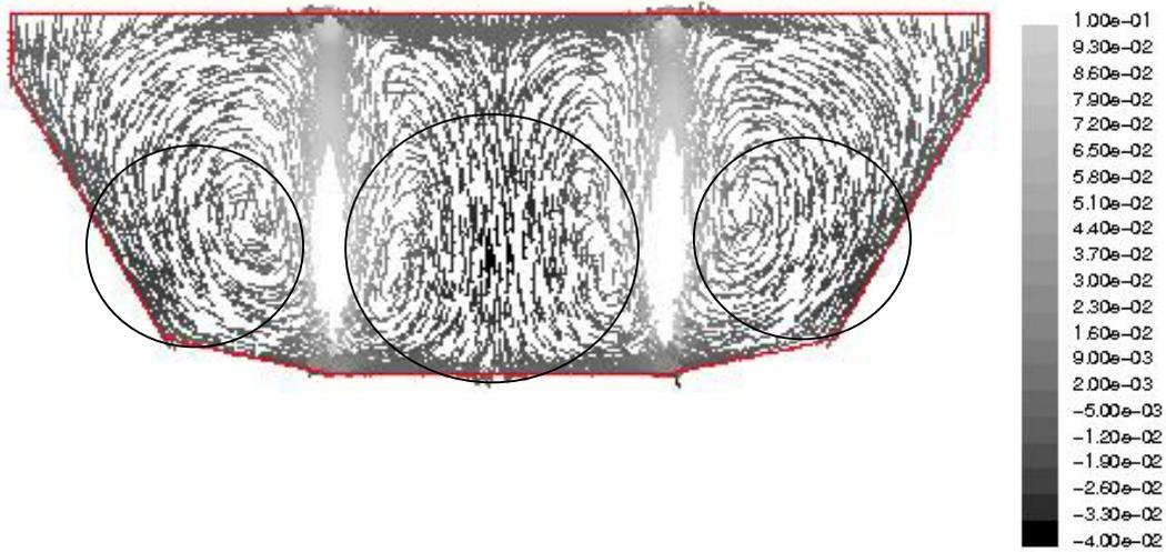
Fig.8 – Velocity field of liquid phase (axis components of velocity)
