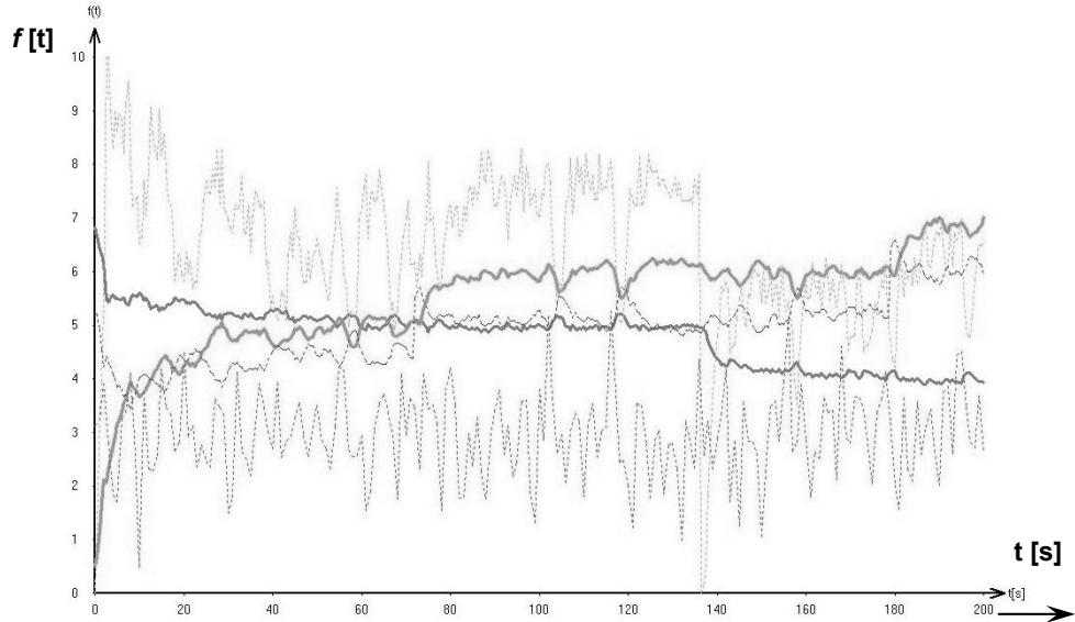
**Fig. 9** The final chart of WinCTRL program module - PID control algorithm with 2 control outputs (temperature of bulb – grey line, flow of air – green line), 2 control input variables (voltages on main ventilator -blue line, on bulb – red line, on second ventilator – violet line).
