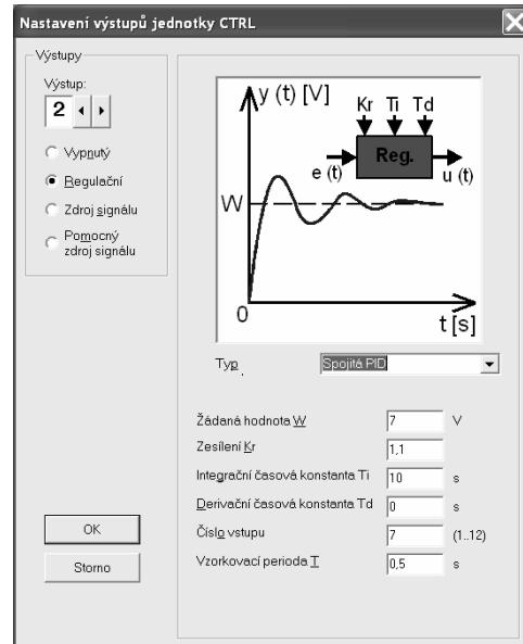
**Fig. 6** Setting of outputs CTRL unit in program module WinCTRL – PID algorithm.
