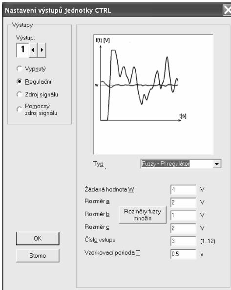
**Fig. 5** Setting of outputs CTRL unit in program module WinCTRL – fuzzy algorithm
