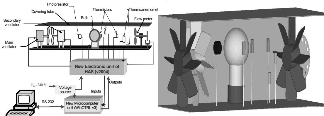
**Fig. 1** Block schema of experimental model HAS (Hot-Air Stand), version 2004
