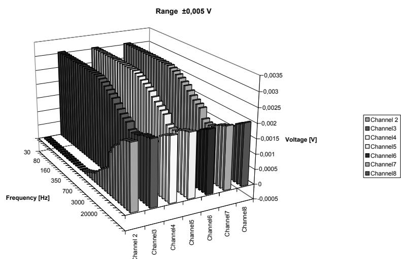
**Fig. 7** The dependency of error on sample frequency
