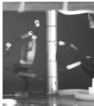
**Fig. 3** Cold tensile test sample
