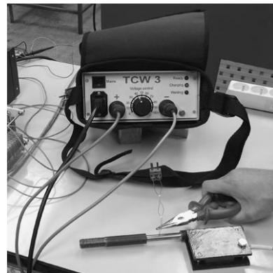
**Fig. 2** Thermocouple welding machine
