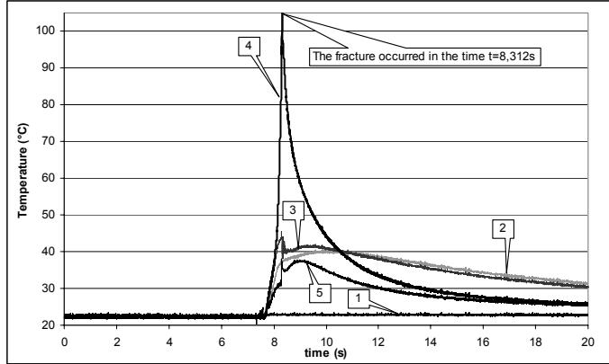
**Fig. 5** Evolutions temperatures were measured with five thermocouples
